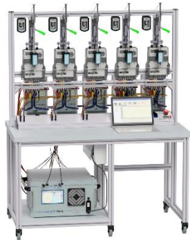
3 phase Test Bench
