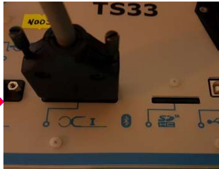
Connect current clamp plug into the socket on TS33. Clamp symbol appears on display.
