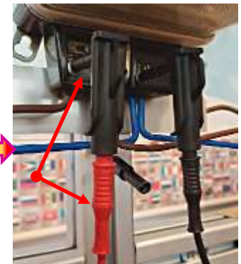
Connect „Phase” meter terminal to phase safety cable by means of magnetic plug
