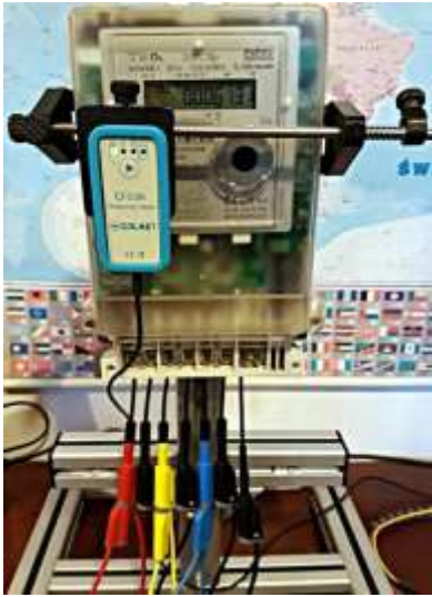
Connected meter ready for testing
