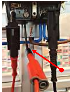
Connect phase current cable to „Cu” pin (red)
