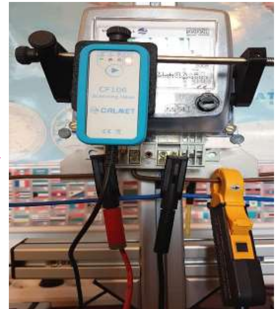
Connect voltage magnetic plugs and assembly the scanning head
