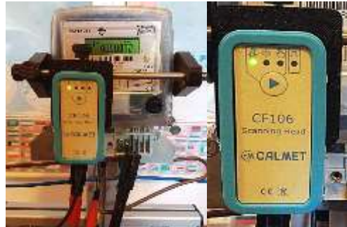
„Click” scanning head and set LED sensing option
